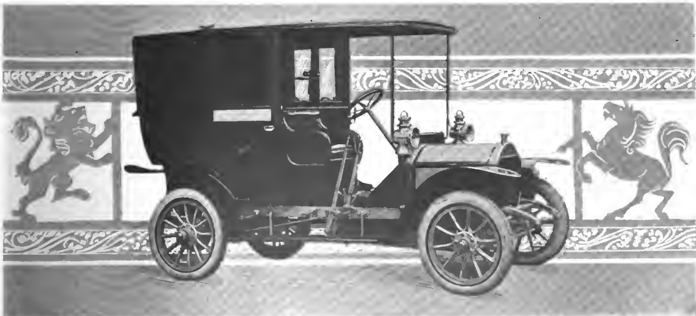
Fig. 6—Napier taxicab and town car model with a wheelbase long enough to make the entrance commodious and chassis low to match.
